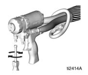
17. Disengage gun piston safety lock.
