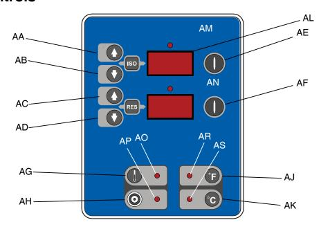
Fig. 2 Heater Controls and Indicators
