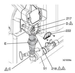
Flat side faces up. Tighten by hitting firmly with non-sparking hammer.
