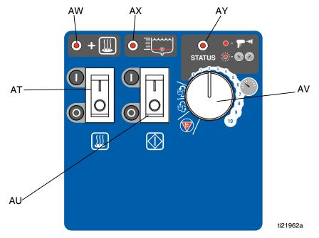
Fig. 3 System Controls and Indicators
