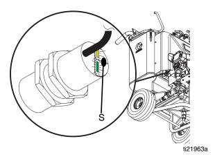
Fig. 22 Adjustment Screw
