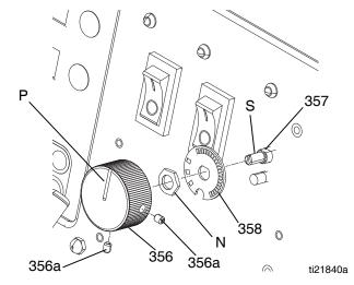
Fig. 9 Function Knob/Potentiometer
