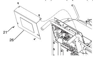
3. Locate the DIP switch on the control board.
