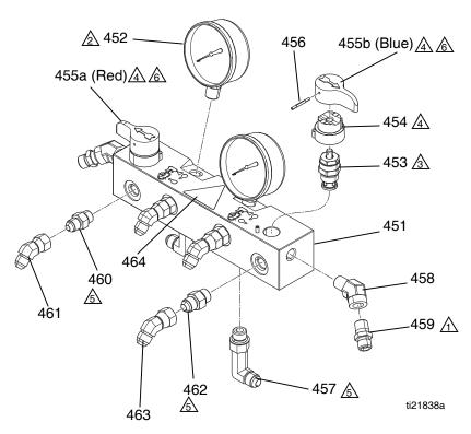
Apply sealant to assembled non-swiveling pipe threads.
