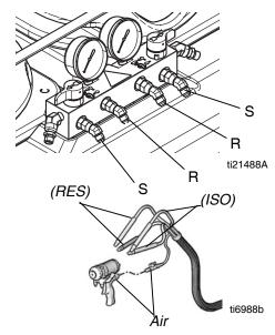
Fig. 5 Connect the Recirculation Hoses
