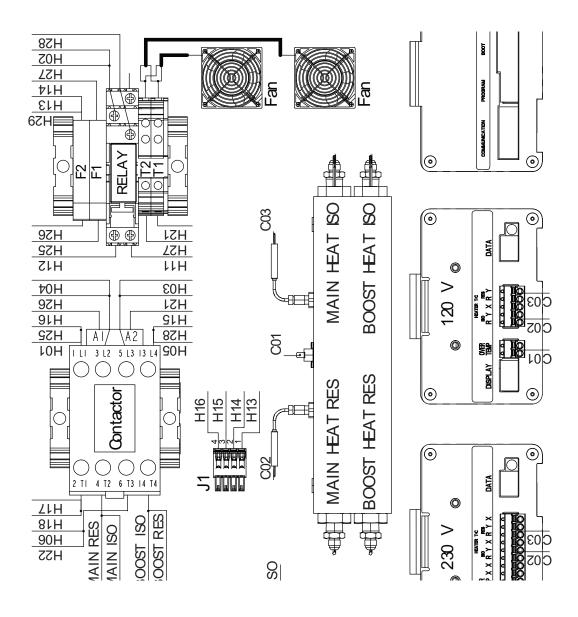
Fig. 23 Power Harness (78) Wire Identification
