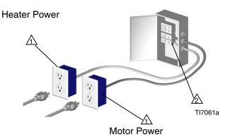
Ensure no other high amp loads are connected while running Reactor.
