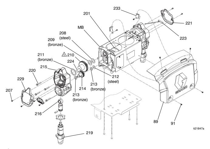
Crankshaft must be in line with crankshaft at other end of motor, so pumps move up and down in unison.
