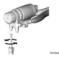
**12.** Disengage piston safety lock.
