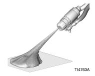
**14.** Apply layer of lubricant over front of gun and lock ring, or use gun cover to prevent overspray buildup and ease disassembly. See Fusion Gun Manual 309856 or 309550 to order lubricant and gun cover
