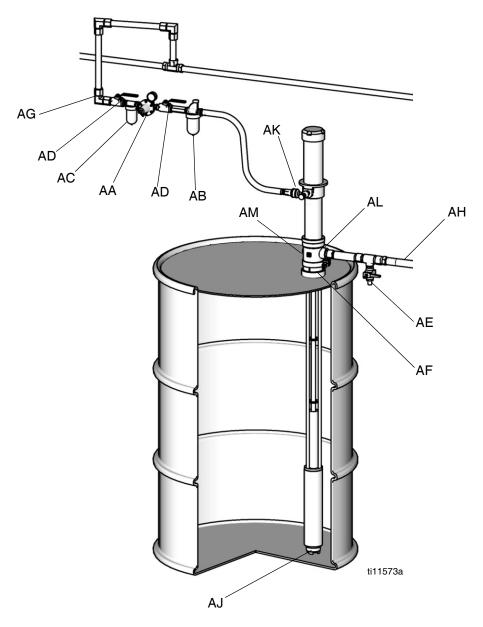
Fig. 3: Typical Installation for Lubrication Applications
