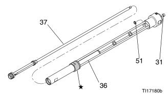
★ Support the Series A, B, and D pump frame with a strap wrench. Series C pumps have wrench flats.
