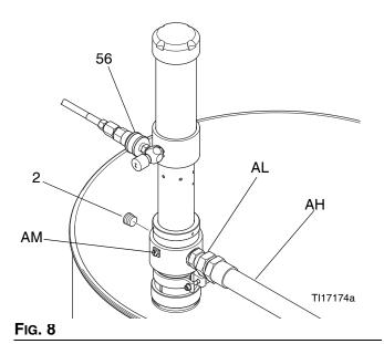
6. Connect a grounded fluid hose (AH) to the 1/2 npt(f) fluid outlet (AL). In a circulating system, remove the pipe plug (2) and connect a fluid return line to the 3/8 npt(f) return port (AM).
