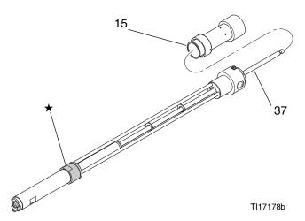
★ Support the Series A, B, and D pump frame with a strap wrench. Series C pumps have wrench flats.
