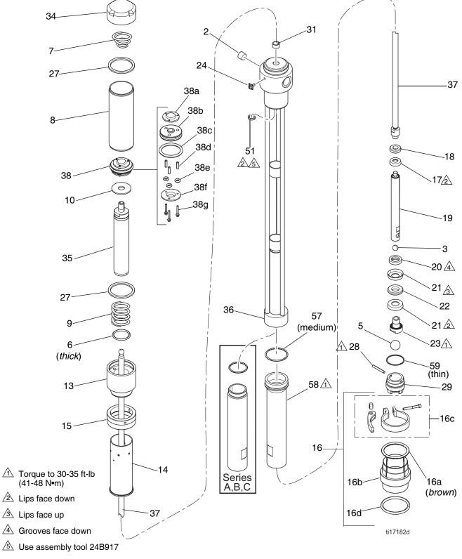
**NOTE:** Thin, medium, and thick refers to the relative cross section thickness of the o-rings.
