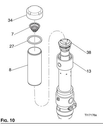
Unscrew the cylinder (8) from the air motor base (13) and lift the cylinder straight off the air piston (38). Unscrew by hand or use a chain wrench to prevent distortion of the cylinder's shape. See Fig. 10.
