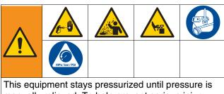
manually relieved. To help prevent serious injury from pressurized fluid, such as skin injection, splashing fluid and moving parts, follow the Pressure Relief Procedure when you stop spraying and before cleaning, checking, or servicing the equipment.
