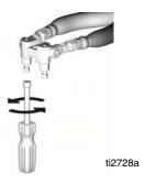
3. Attach gun fluid manifold. Connect gun air line. Open air line valve.
