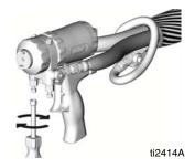
17. Disengage gun piston safety lock.
