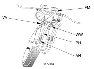
**NOTE:** Manifold hose fittings (VV, WW) allow use of 1/4 in. and 3/8 in. ID Reactor heated fluid hoses.
