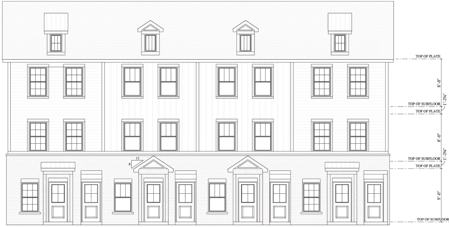
ELEVATION - FRONT SCALE 1/4" = 1'-0"
